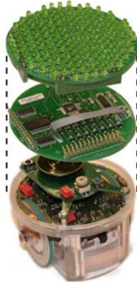
Fig. 4. The two printed circuit boards of the see-Puck module are mounted on top on an e-Puck.
