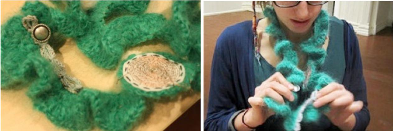
Fig 2. The use of textile and soft materials guided the way the *Speaker Scarf* has been designed, in particular the specific physical manipulations that need to be performed in order to listen to the music. Left: the textile speaker unit and the on/off switch that can be also used for adjusting the volume. Right: Adjusting the volume by placing a metallic button on one of the loops made of resistive yarn.
