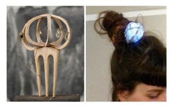
Figure 6: Prototype of the wooden bling hair needle made of wood, hand painted silk fabric, conductive thread, LEDs and an accelerometer.
