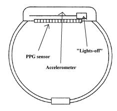
**Fig. 5.1.** Scheme of a proposed wrist sensor with a PPG sensor capable of measuring Blood Volume Pulse, a triaxial accelerometer and a "lights off" switch.
