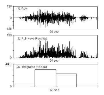
**Fig. 4.1.** Post processing of accelerometer. 1) Raw counts; 2)Rectified counts; 3) Epochs. Extracted from (Chen & Basset 2005)
