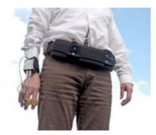
Fig. 4.12. Usage of Portapres. The sensors in the wrist and fingers communicate with the belt which has data storage capacity and a power source
