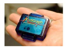
Fig. 4.2. Actigraph, an example of an accelerometer.
