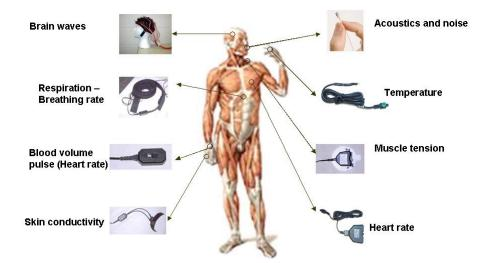
**Fig. 2.9.** Examples of usual places in the body used to capture signals from wearable sensors. Some of this signals will be discussed along this thesis. Adapted from (Kim 2004)
