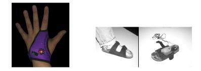
Fig. 4.7. Example of skin conductivity sensors in the hand and in the foot. Extracted from (Picard & Scheirer 2001) and (Picard & Healey 1997)
