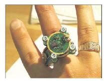
Fig. 2.6. Early prototype of a PPG ring
