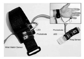
Fig. 4.11. Wearable sensor for measuring blood pressure through PPT method. It is composed of two PPG sensors.
