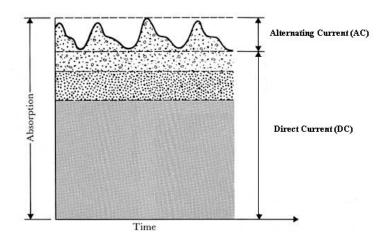
Fig. 2.7. Absortion of light by a PPG sensor. The AC part of the signal gives information about the heartbeat
