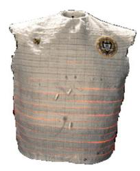
Fig. 2.8. Example of a smart textile called Georgia Tech Wearable Motherboard  $^{\text{TM}}$
